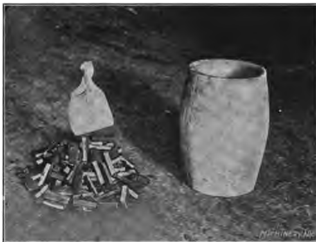
Fig. 1. Charge for Making Crucible Steel, consisting of Swedish Iron, a Bag of Charcoal, and the Clay Crucible in which the Charge is melted
